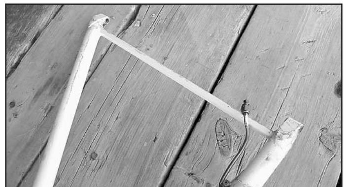
*Square tubing installed in place of the fabric former.*
