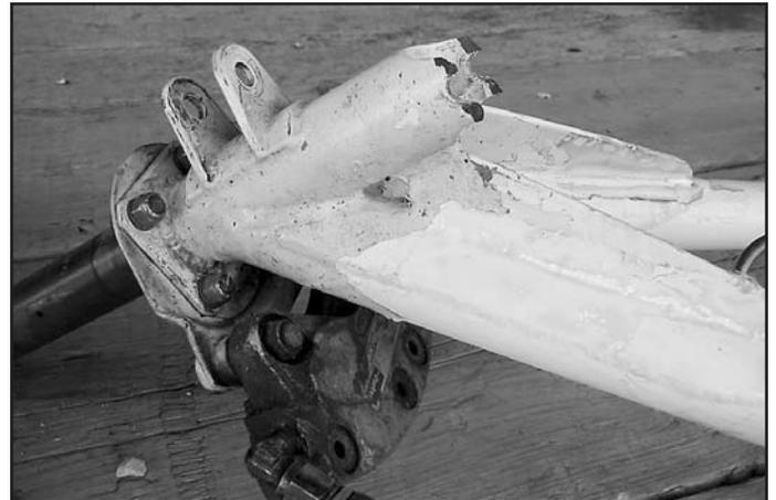
*A heavy duty gear with the shock strut mounts tore off the end of the axle.*
