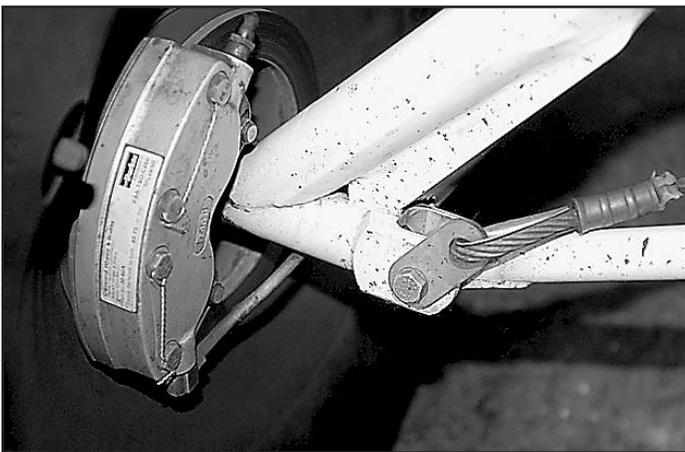
*Cub Crafters heavy duty gear with machined axle/shock strut mounts.*
