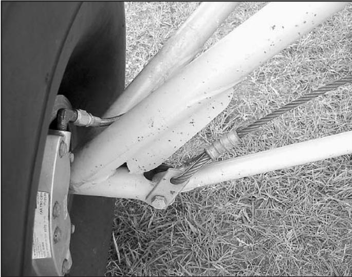
*Large gussets and sleeves on a heavy duty gear.*
